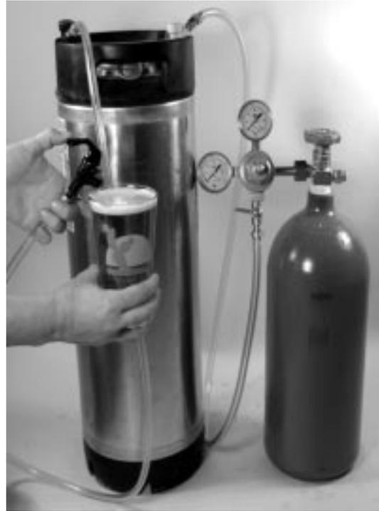
Many times the O-ring will not seal if you initially pressurize to only 10-15 psi. Initially overpressurize to seat the lid o-ring and then you may back off the pressure and the lid will remain sealed. Lubricate the O-ring with food grade silicone (see catalog page 17) to greatly facilitate sealing. Use water if you don't have silicone.
